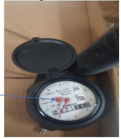
Both of these meters has a "snowflake". When the "snowflake" is turning there is water passing through the meter. If you think you have a leak turn off all your water and check to see if the "snowflake" is still turning.
